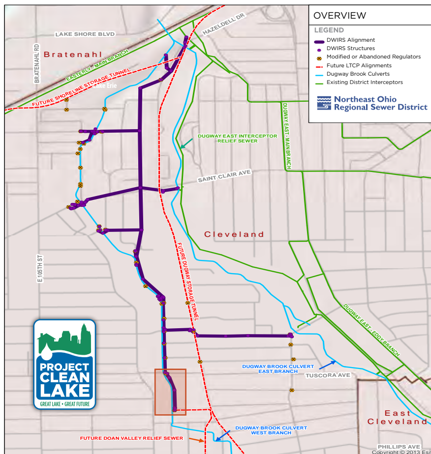
Project Clean Lake plan overview of DWIRS with location of curved microtunnel segment highlighted. Southern end runs close to existing culvert (courtesy NEORS)
