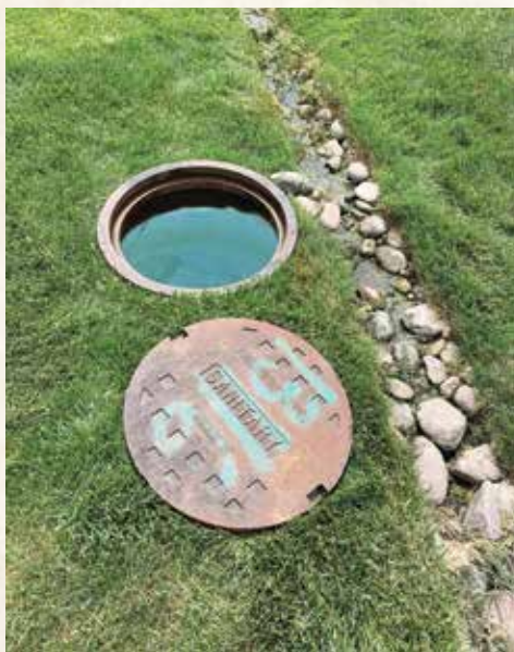
Green fluorescent dye was used to simulate the dyed water testing that was originally used to identify the failing laterals
