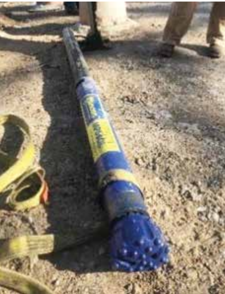
Mincon rock hammer pilot head
