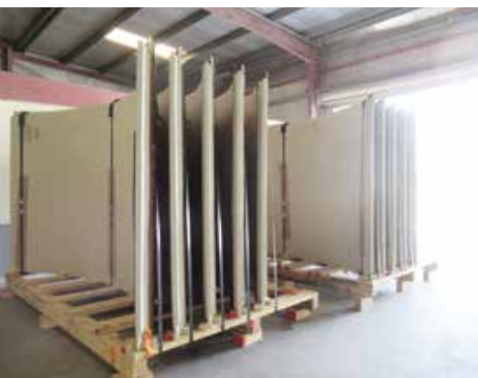
Proprietary system offered a way to break the geometrically complex pipe liners down into multiple component segments to dramatically reduce shipping costs, while still maintaining structural integrity and load capacity
