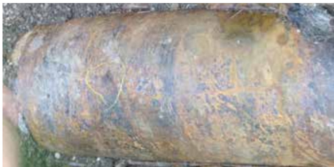
Figure 5. Leak discovered at Site 2 – Gas Pocket 1 during the BEM inspection
