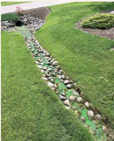
Green fluorescent dye was used to simulate the dyed water testing that was originally used to identify the failing laterals
