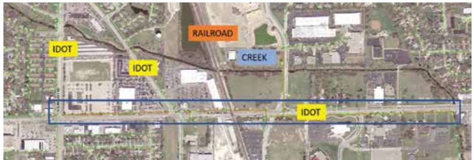
Alignment located in IDOT ROW, with crossings at a railroad and a creek
